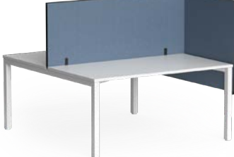
Height 578mm; 1300mm AFL Uses aluminum screen joiners to spine screen and high-strength adhesive to worktop.
